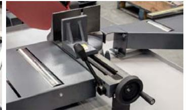
Connection of the left and right roller conveyor - detail
