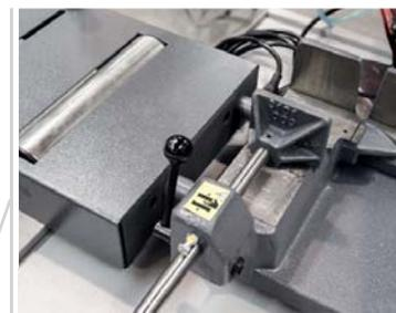
Connection of the inlet roller conveyor - detail
